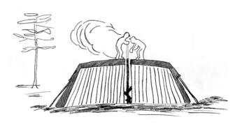
**Figure 10.2:** A cross-section of a charcoal stack that is lit at the centre. The timber is placed standing on end and is then covered with earth and brushwood to prevent the air-flow. Illustration: Fia Johannessen.
